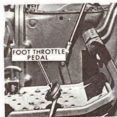
Figure 5 Foot Throttle—Ford 2110 and 4110
