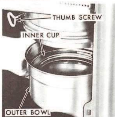
Figure 84 Air Cleaner—Oil Bath Type
