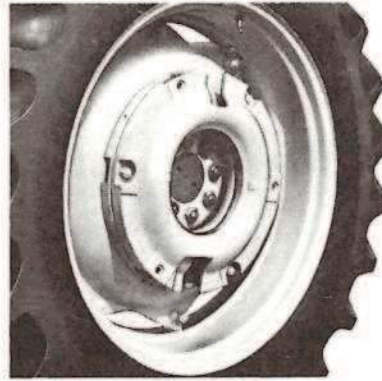
Figure 66 Rear Wheel Weights—Ford 2000, 3000, 4000, 4000 SU and 5000
