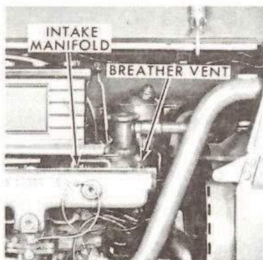
Figure 109 Breather Vent—Ford 5000 Gasoline
